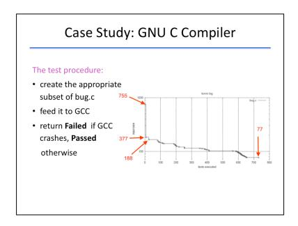
We next write the test procedure to be provided to the delta debugging algorithm. This procedure consists of three steps. First, it creates the appropriate subset of bug.c. Next, it feeds this subset to GCC. Finally, it returns Failed if GCC crashes, and Passed otherwise.
