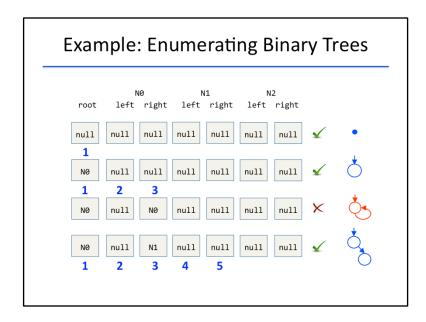
This algorithm is a rather abstract manipulation of data structures, so let's take a look at how Korat would work in a concrete example to get a better idea of what it is doing. Let's see how Korat would generate test cases for a BinaryTree object with three Nodes.
